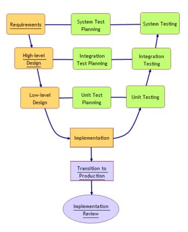
Figure 14.7 Example of Software Development Using V-Methodology
