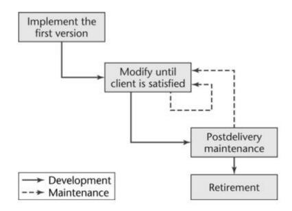
Figure 13.5 Maintenance Requirements in Code and Fix
